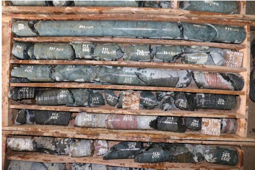
Figure 1: Drill cores NamXe South, host rock NG (grey) and Red ore ROE (reddish)
