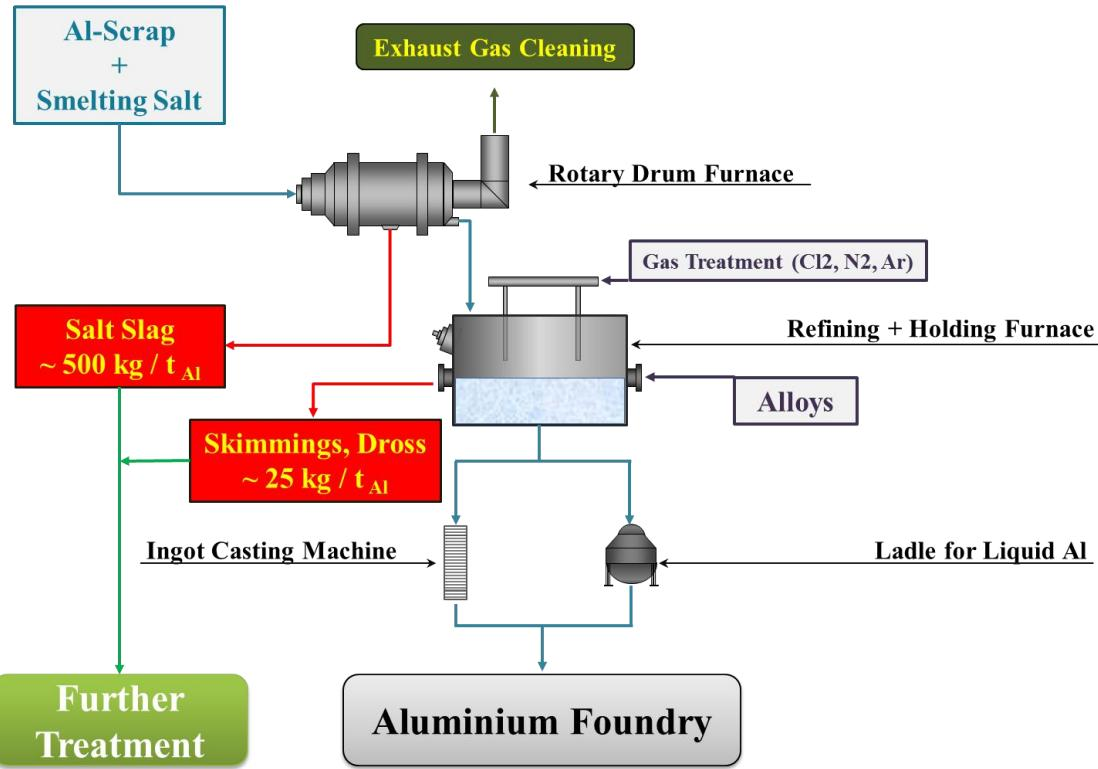
Rotary melting furnaces are used to melt down the aluminium scrap and other materials containing Al. Typical melting rates vary from 0.5 - 3.0 t/h. The melt process is carried out under a layer of salt, which absorbs the oxides and impurities from the scrap and protects the aluminium melt from oxidation loss (burn-off).
