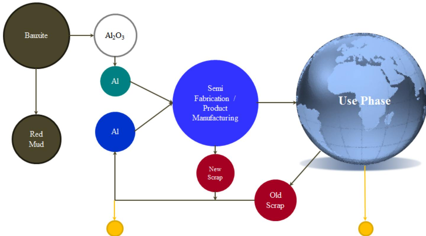
The share of recycled aluminium metal will increase steadily. The amount of Aluminium “stored” in use, will not increase (no net addition). The Primary Al, will just be used to equal the losses during collecting, processing and refining of old scrap and collecting and re-melting of new scrap. To avoid environmental damages, the residue free reclamation of the growing amount of residues has to be implemented all over the world.
