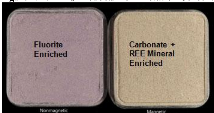
Figure 1: WHIMS Products from Flotation Concentrate (Test 3612-117)
